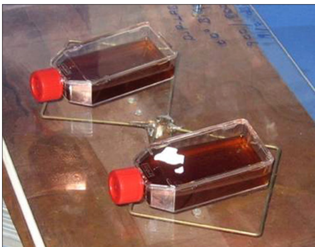
Fig. 1. The biquad antenna and the placement of samples.
